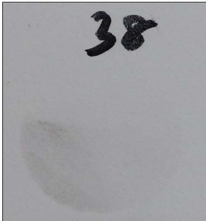
Chemical spot test #38, Sodium Hydroxide (20%), Rating 2, Color change
