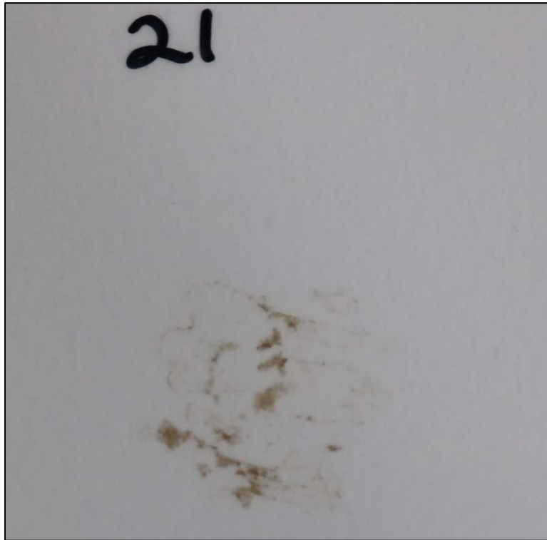
Chemical Spot Test #21, Furfural, Rating 2, Staining
