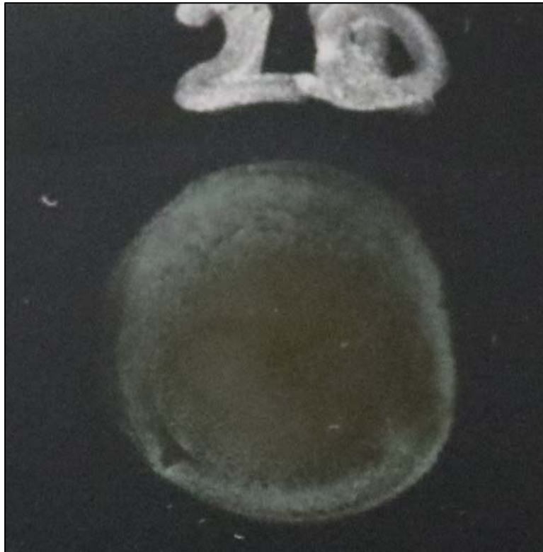
Chemical Spot Test #20, Formic Acid (90%), Rating 2, Gloss change (Staining occurred by residual flow form chemical spot test #26, tincture of iodine, during rinsing.)
