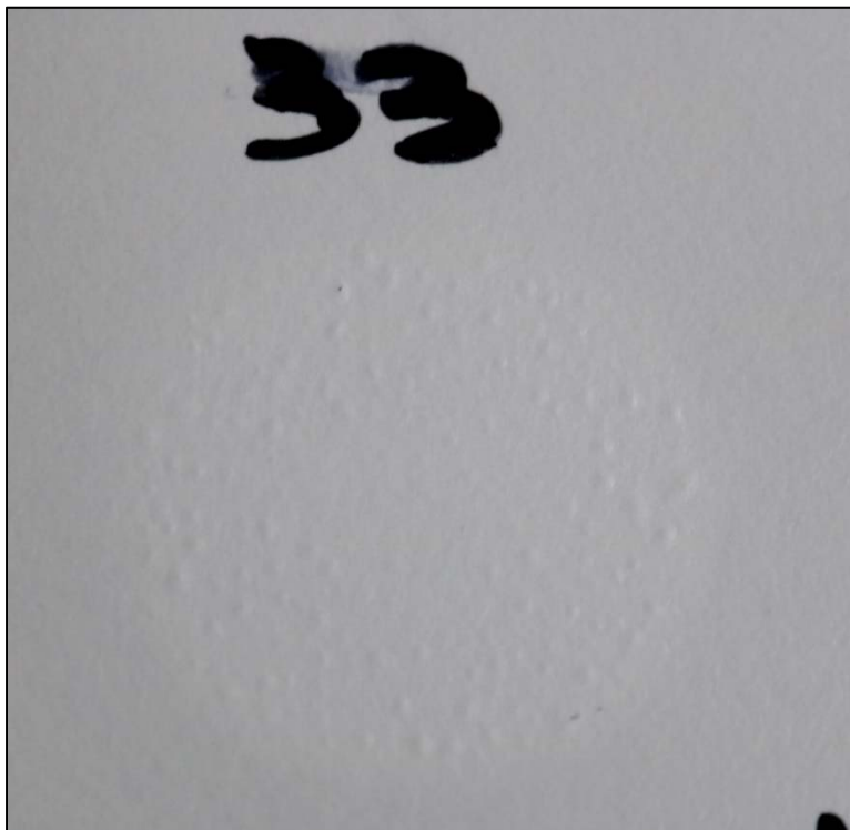
Chemical spot test #33, Nitric Acid (70%), Rating 3, Surface swelling
