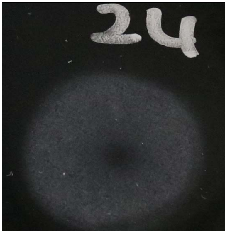
Chemical spot test #24, Hydrofluoric Acid (48%), Rating 2, Gloss change
