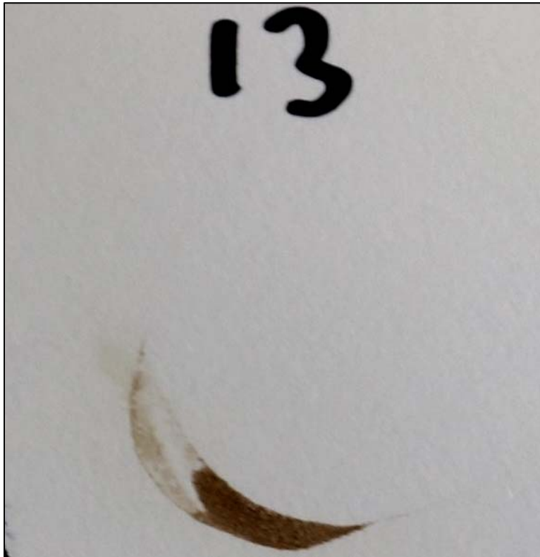
Chemical spot test #13, Chromic Acid (60%), Rating 2, Staining
