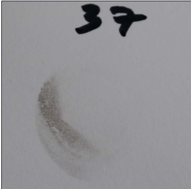
Chemical spot test #37, Sodium Hydroxide (10%), Rating 2, Staining, color change
