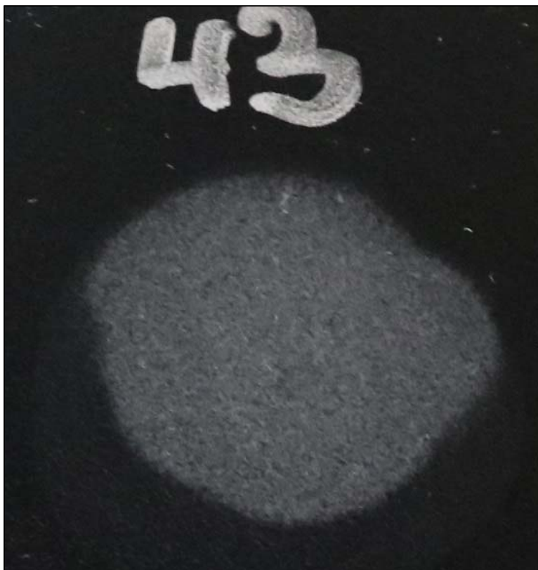
Chemical spot test #43, Sulfuric Acid (77%), Rating 2, Gloss change
