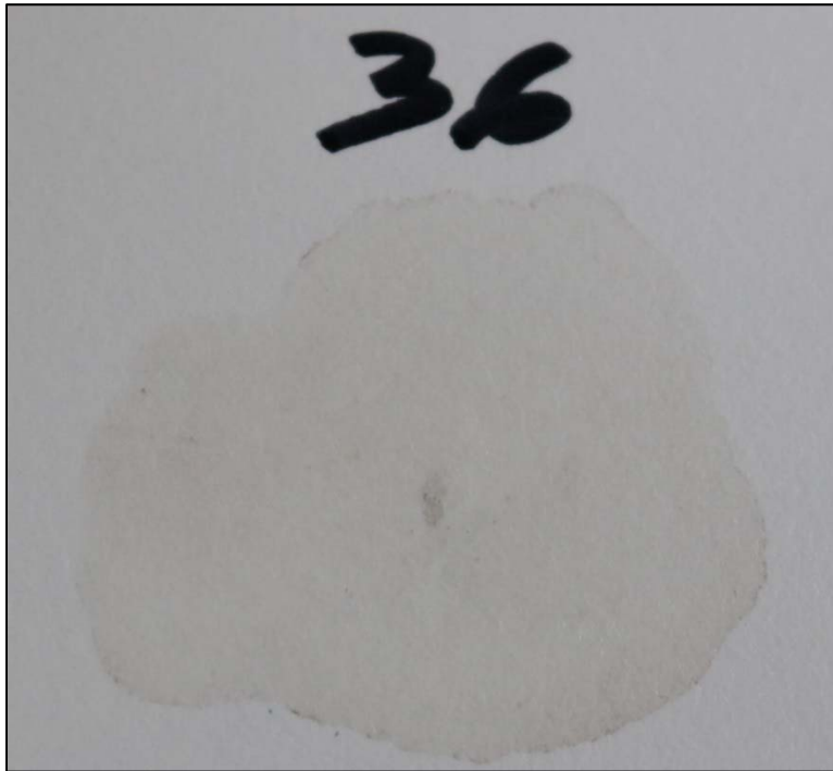
Chemical spot test #36, Silver Nitrate, Saturated, Rating 2, Staining, color change
