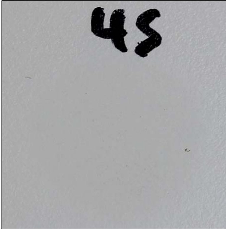
Chemical spot test #45, Sulfuric Acid (77%) and Nitric Acid (70%), equal parts, Rating 2, Gloss change
