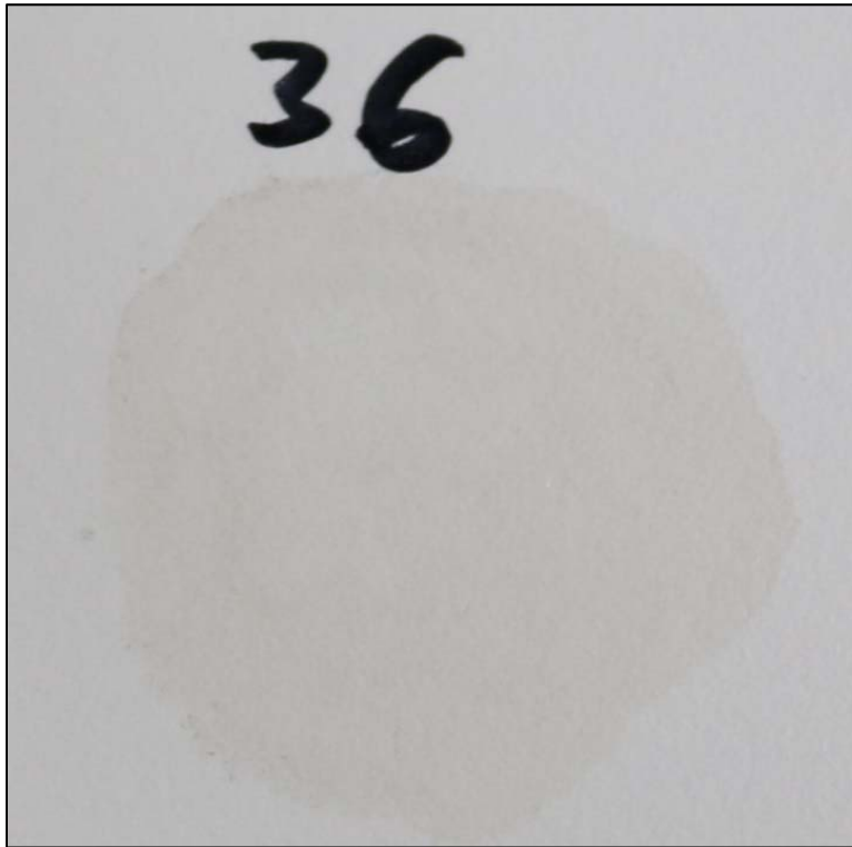
Chemical spot test #36, Silver Nitrate, Saturated, Rating 2, Staining, color change
