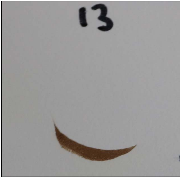
Chemical spot test #13, Chromic Acid (60%), Rating 2, Staining
