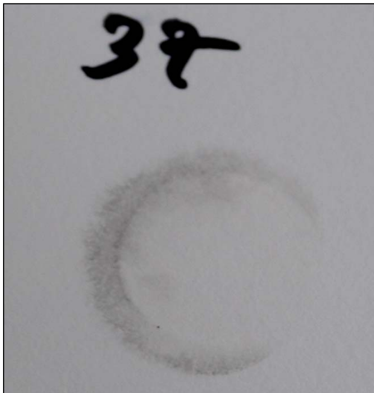
Chemical spot test #37, Sodium Hydroxide (10%), Rating 2, Staining, color change
