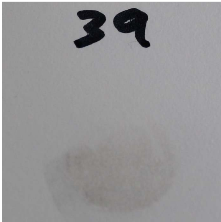
Chemical spot test #39, Sodium Hydroxide (40%), Rating 2, Staining, color change
