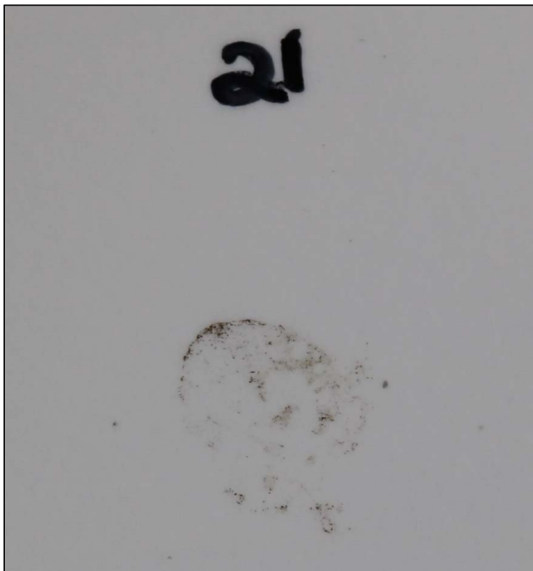
Chemical spot test #21, Furfural, Rating 2, Staining
